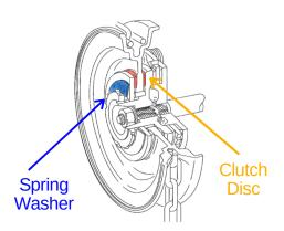
The hand wheel is equipped with a special Belleville washer and clutch disc. When the pulling force on the hand chain exceeds the limit, the clutch will slip and the force will not be transmitted to the load sprocket. The hoist will not lift the load.
