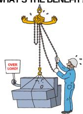
This unique feature protects the hoist from damage in the event of an unexpected overload, thereby ensuring safety during lifting.
