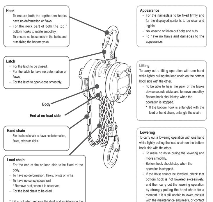
\* If it is not oiled, remove the dust and moisture on the load chain and apply the lubricant JIS K 2246 class 1, No.1 (code: NP-9) rust preventive oil equivalent (DAPHNE OIL COAT RL-44, IDEMITSU KOSAN Co., LTD. recommended) Consult KITO if the usage environment does not allow the application of lubricating oil to the load chain.
